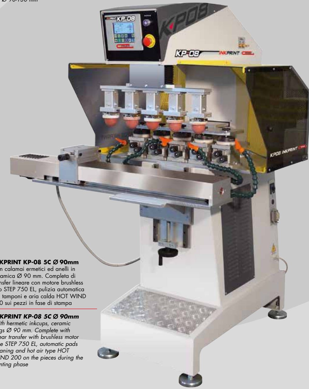
HERMETIC INKCUPE INKPRINT KP-08 works with hermetic inkcups and ceramic rings of Ø 90-130 mm
